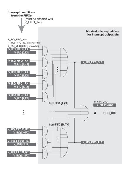
Figure 12.7: FIFO interrupt
