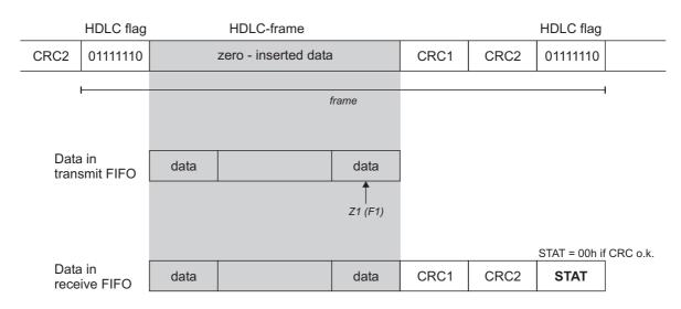
Figure 4.2: FIFO data organization in HDLC mode
