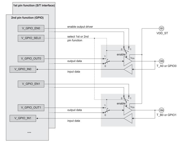
Figure 13.2: GPIO block diagram (GPIO0 and GPIO1 exemplarily)
