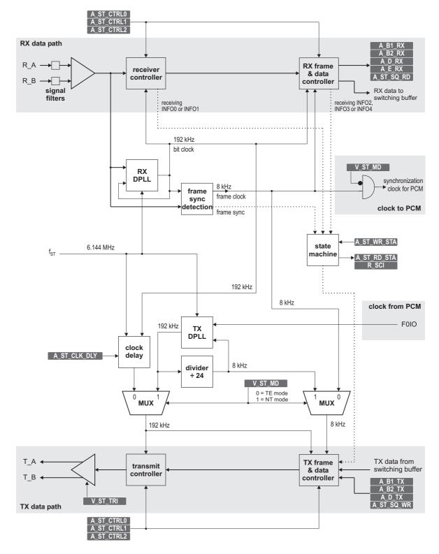
Figure 5.3: Block diagram of the S/T interface module
