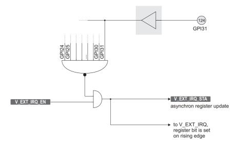
Figure 12.9: External interrupt block diagram
