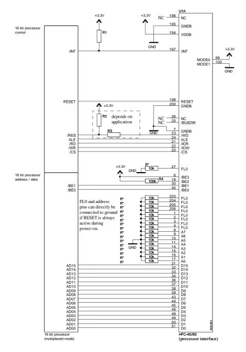
Figure 2.20: 16 bit Intel processor circuitry example, mode 4, multiplexed
