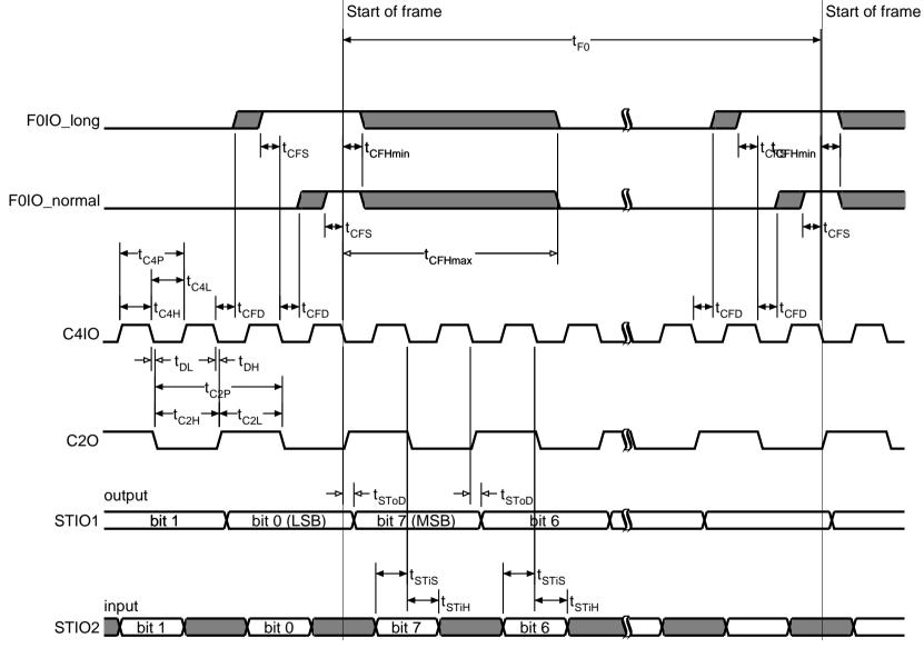
STIO1 is shown as data output and STIO2 as data input. However, both pins can change their I/O characteristic with every PCM time slot.
