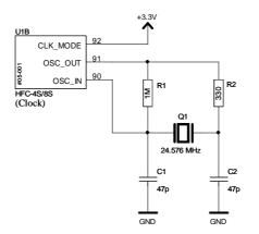
Figure 12.2: Standard HFC-4S/8S quartz circuitry
