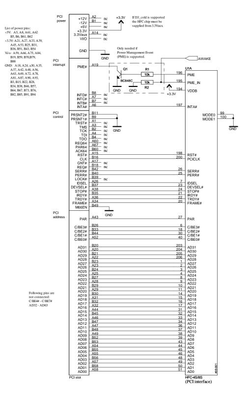
Figure 2.6: PCI connection circuitry
