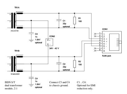
**Figure 5.14:** Transformer and connector circuitry in NT mode (shown with optional 100 $\Omega$  termination, whole bus termination must be 50 $\Omega$ )
