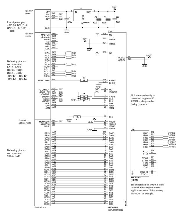
Figure 2.7: ISA PnP circuitry, see Section 2.4.1 on page 62 for IRQ line assignment
