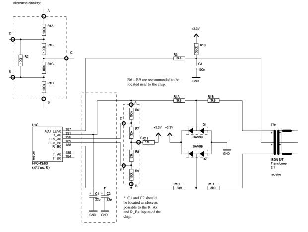
Figure 5.9: External S/T receive circuitry for TE and NT mode
