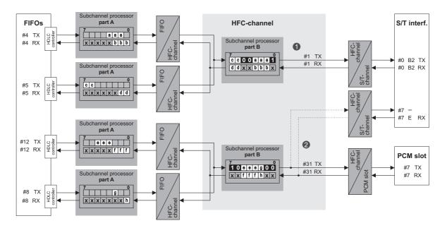
Figure 3.18: CSM example with subchannel processor
