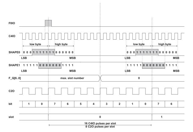
Figure 6.7: Example for two CODEC enable signal shapes with SHAPE0 and SHAPE1.
