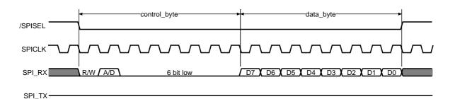
**Figure 2.21:** *SPI write transaction*  $(R/\overline{W} = '0')$
