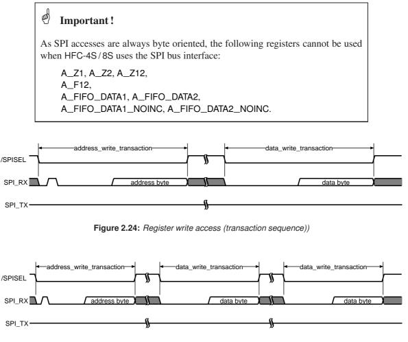
Figure 2.25: Multiple write access to the same register
