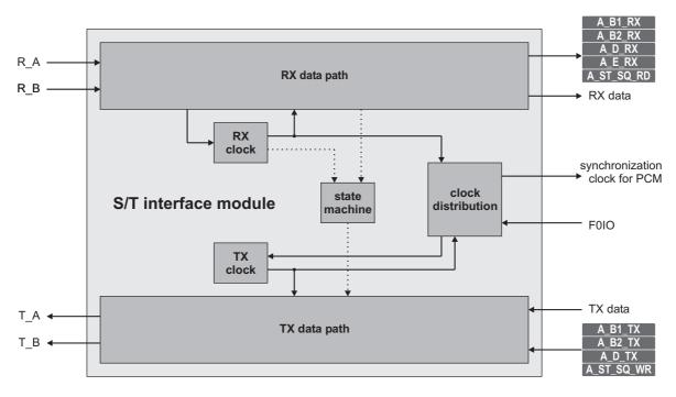
Figure 5.1: Overview of the S/T interface module
