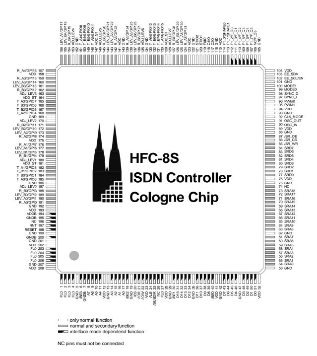
Figure 1.6: HFC-8S pinout in parallel processor mode
