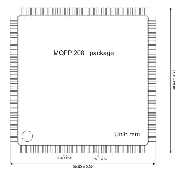
**Figure 15.1:** *HFC-4S/8S package dimensions*
