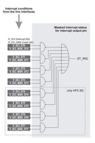
Figure 12.5: *S*/*T* interface interrupt
