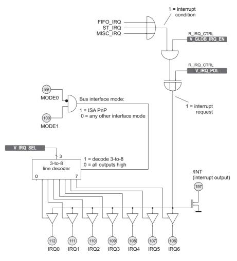
Figure 12.4: Interrupt output
