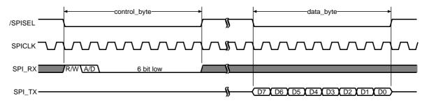
Figure 2.23: Split SPI read transaction
