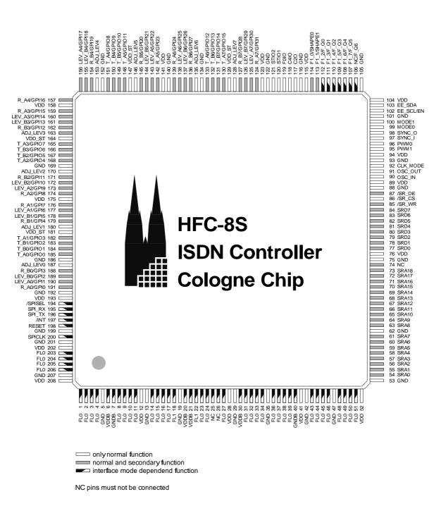
Figure 1.7: HFC-8S pinout in SPI mode
