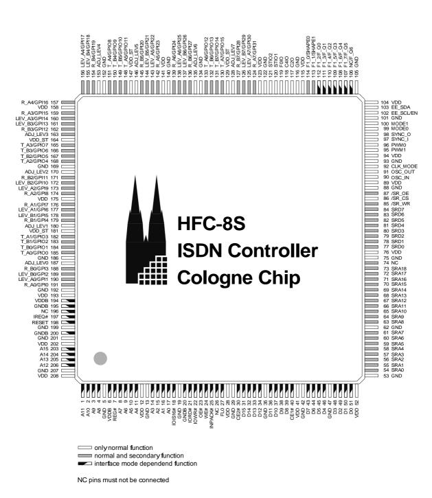
Figure 1.5: HFC-8S pinout in PCMCIA mode
