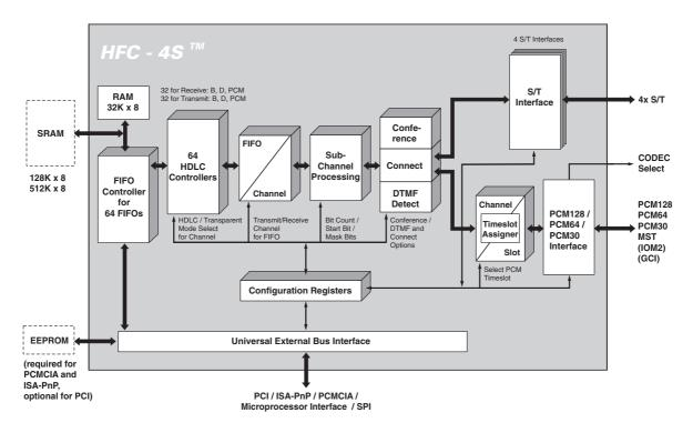
Figure 1.2: HFC-4S block diagram
