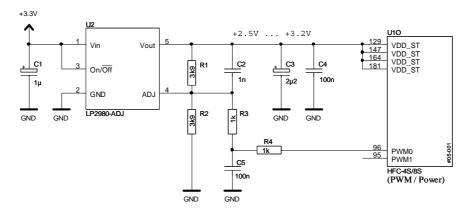
Figure 5.12: VDD\_ST voltage generation
