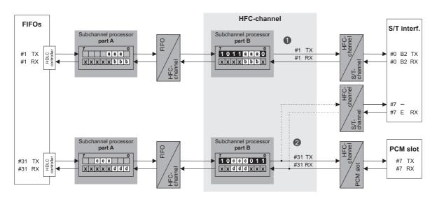
Figure 3.17: SM example with subchannel processor
