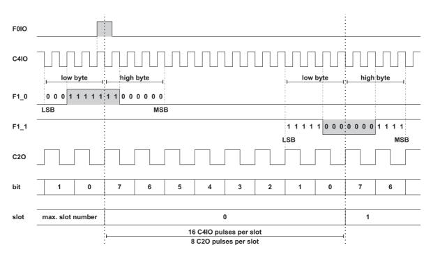
Figure 6.6: Example for two CODEC enable signal shapes
