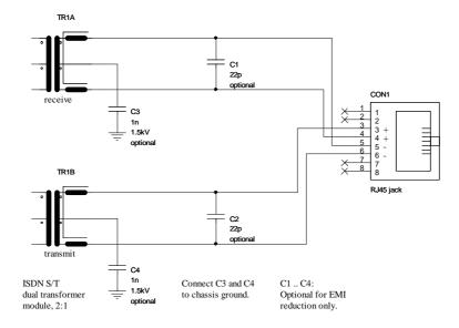
Figure 5.13: Transformer and connector circuitry in TE mode
