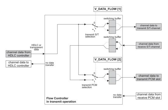
Figure 3.3: The flow controller in transmit operation
