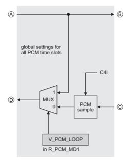
Figure 6.2: Global settings for all PCM time slots (detail of Figure 6.1), normally used for test loop setup
