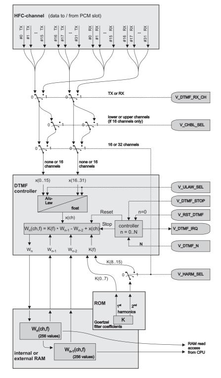
Figure 9.1: DTMF controller block diagram
