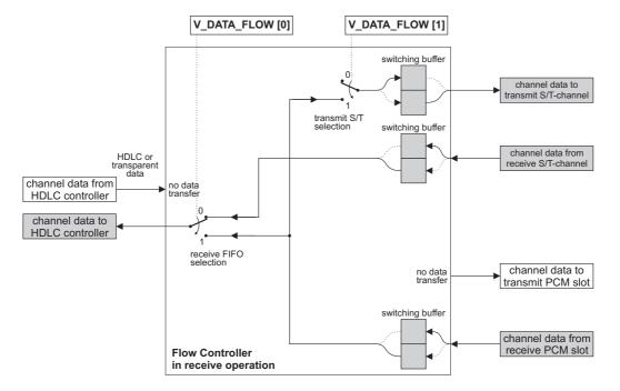
Figure 3.4: The flow controller in receive FIFO operation
