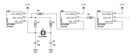
Figure 12.3: Cascade-connected HFC-4S/8S with only one quartz circuitry
