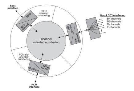
Figure 3.2: Areas of FIFO oriented, HFC-channel oriented and PCM time slot oriented numbering
