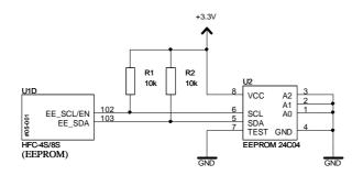
Figure 2.1: EEPROM connection circuitry
