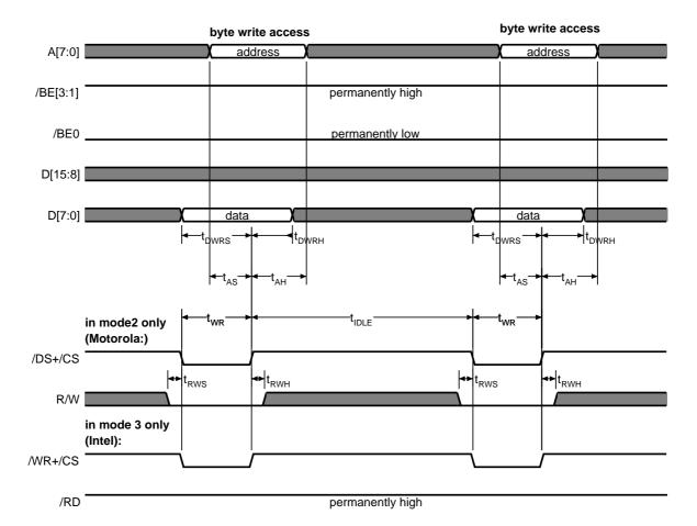
Figure 2.10: Write access from 8 bit processors in mode 2 (Motorola) and mode 3 (Intel)
