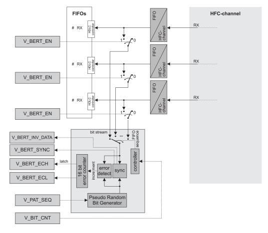
Figure 10.2: BERT receiver block diagram
