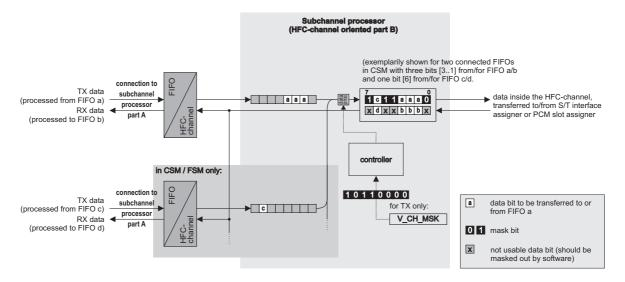
Figure 3.16: Part B of the subchannel processor
