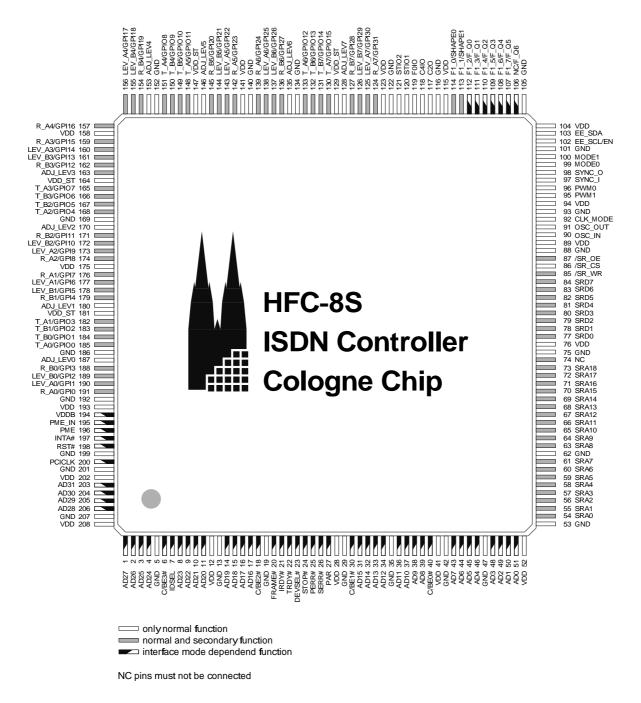
Figure 1.3: HFC-8S pinout in PCI mode
