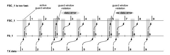
**Figure 5.7:** Data transmission with  $f_{FSC | 1} > f_{FSC | 0}$  (i.e. too fast FSC from unsynchronized TE)
