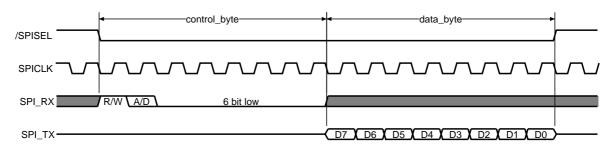
**Figure 2.22:** *SPI read transaction* ( $R/\overline{W} = '1'$ )
