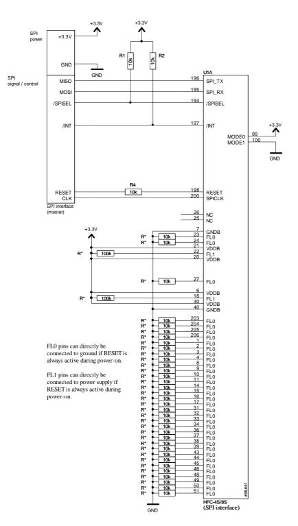
Figure 2.28: SPI connection circuitry
