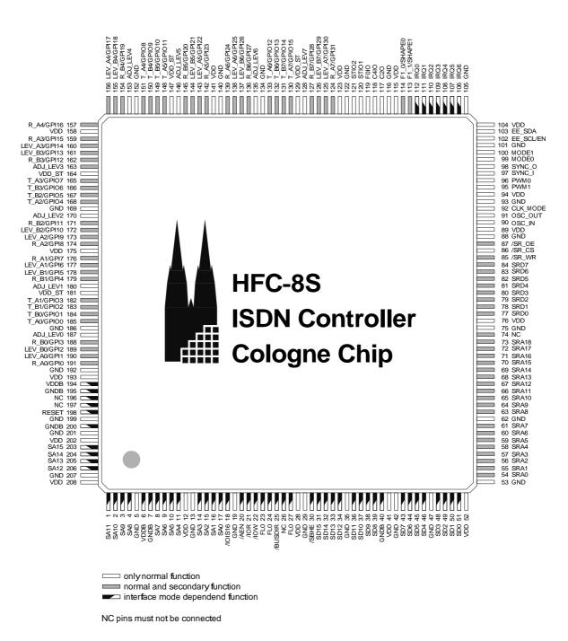
Figure 1.4: HFC-8S pinout in ISA PnP mode
