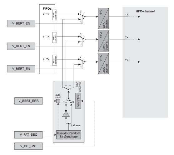
Figure 10.1: BERT transmitter block diagram
